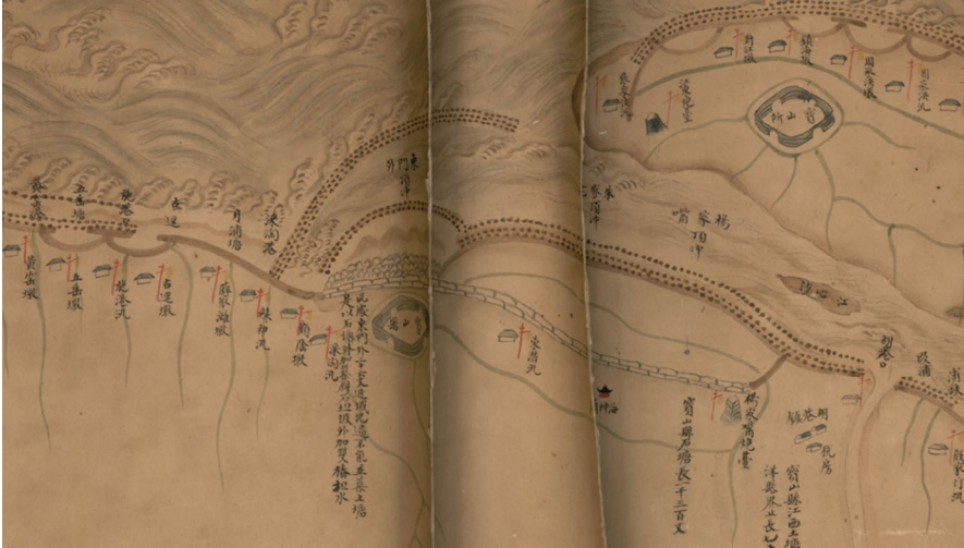
Fig. 14 Detail from “Jiangnan hai tang tu” 江南海塘图 [Map of the Jiangnan Seawall], drawn between 1750 and 1753. There were three lines of a combined sea dike system at the critical intersection between the Yangzi River and the Huangpu River. The strongest and most costly part was the stone levee, outside of which there was an earthen dike. On the seaward side of the earthen dikes, there were several lines of wood piles. When the stone levee abutted the water directly because sufficient space was lacking to build an earthen dike, a stone slope, supported by two lines of wood piles, was built on the waterside. (Library of Congress (call number G7823.J48N22.1795.S6, Vault Shelf AACR2); https://www.loc.gov/resource/g7823j.ct003416/ , accessed 17 October 2017)
