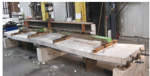
Fig. 11 Final deflected shape of slab 1-C-70
