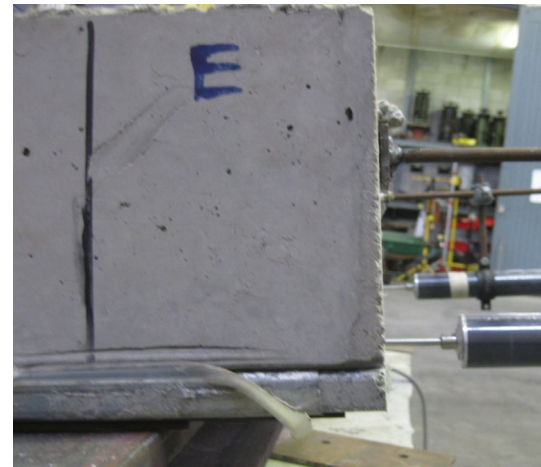
Fig. 6 Final end slip at eastern end support of slab 2-C-70 ( S = 25 mm)
