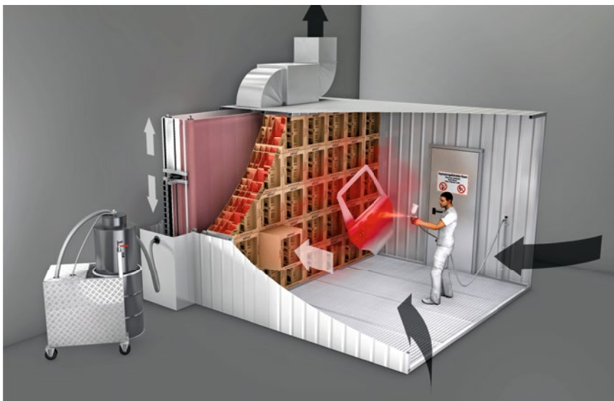
The majority of the overspray is removed by the filter cubes. The circulation filter fleece behind them functions as an after filter. The fine dust trapped by the fleece is continuously transported to the dust collector (left).
