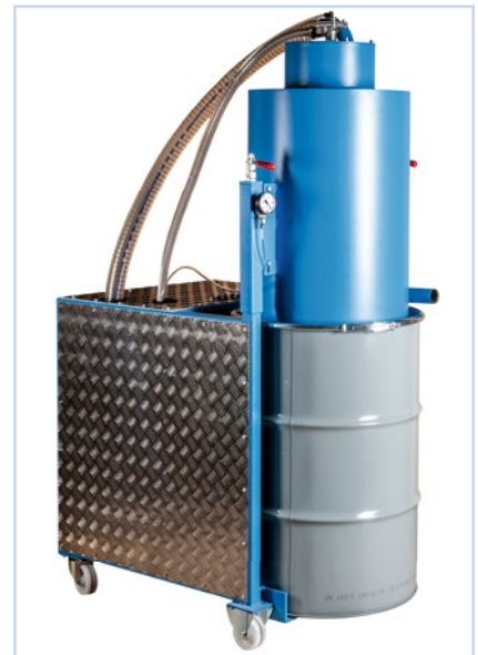
The self-cleaning dust collector extracts the dry paint from the circulation filter fleece and collects it in a 200-litre tank.
