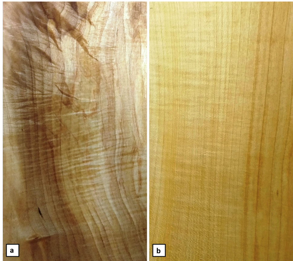
Fig. 5 Wood samples of Acer pseudoplatanus . a Sample 1.1 of plus tree clone Me6 with “high” amount of wavy grain in mature wood. b Sample 10 A (progeny of Me10) with also “high” amount of wavy grain in juvenile wood
