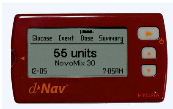
Fig. 1 Example of d-Nav device. The Diabetes Insulin Guidance System has been designed to optimize patients' insulin dosage regimens through the use of algorithms that identify patterns in time-lagged glucose readings and adjust insulin dosage accordingly. This is achieved using a handheld device (d-Nav), which is shown here, and is supported by a nurse-based service to ensure good use
