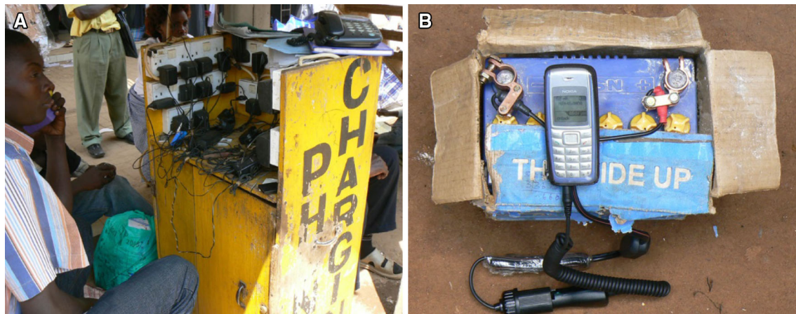
Fig. 1 a Mobile phone charging station, Uganda; b car battery village phone charger, Uganda
