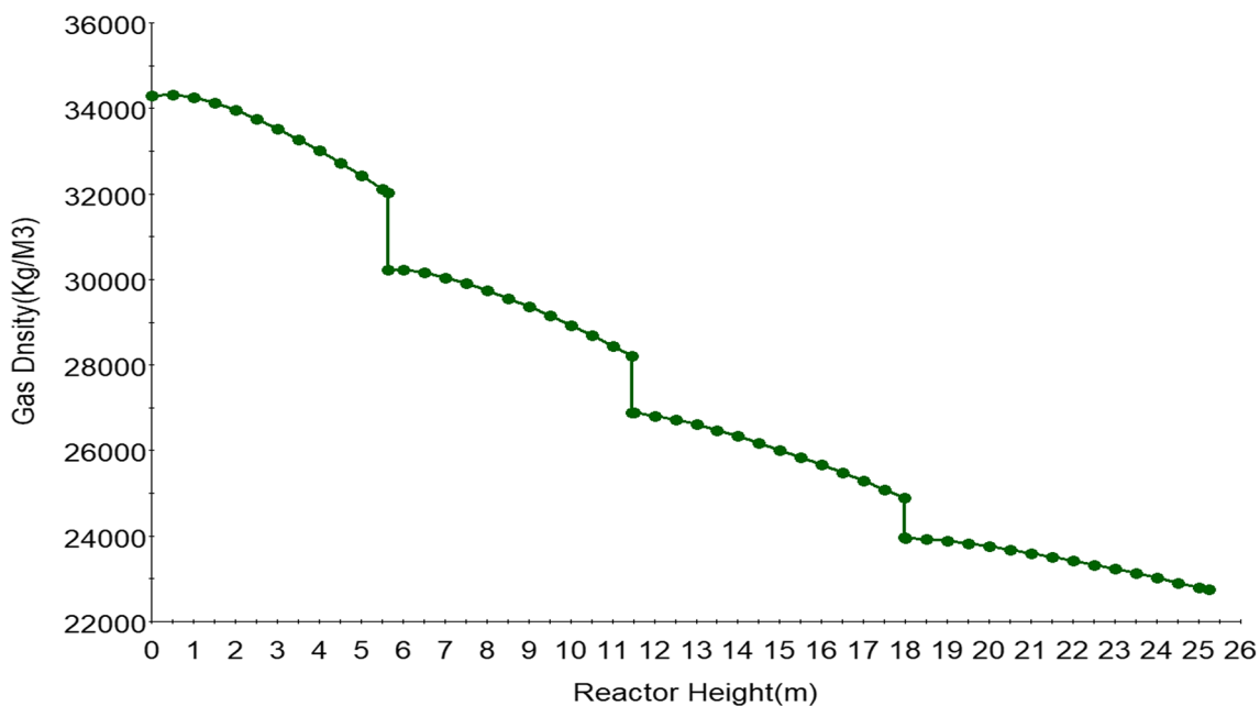
Fig. 11 Gas density profile with changing reactor height
