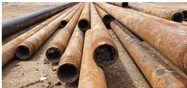
Fig. 1 Cross section of a 90% waxed tubing (Picture courtesy Lease Operators Limited)
