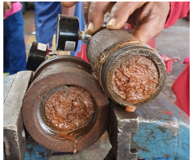
Fig. 9 Cross-sectional view of the chamber containing condensate soaked plugged packed sand after testing
