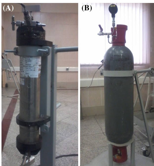
Fig. 4 Experimental samplers: 700-ml liquid sample bottle (a) and 20,000-ml high-pressure gas sample cylinder (b)
