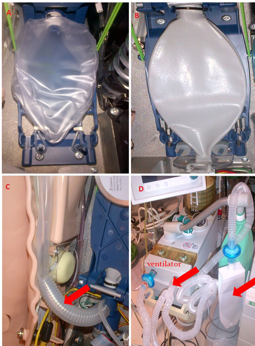
Figure Mannequin modifications to improve mechanical ventilation fidelity A) The stock Laerdal SimMan® 3G mannequin has 350-mL reservoir bags, part 212-11150. B) Modification of the Laerdal SimMan® 3G mannequin with 500-mL Rusch ventilator test lungs,
