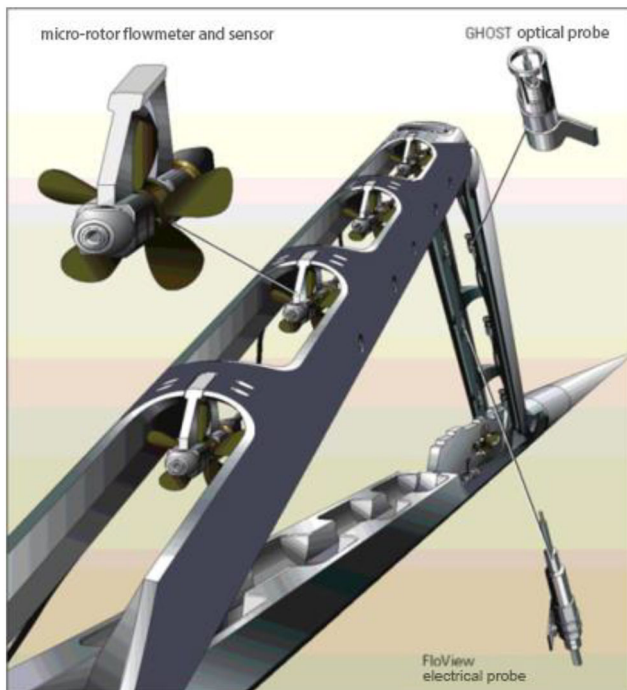
Fig. 2 The fluid scanning imaging logging tool (FSI)
