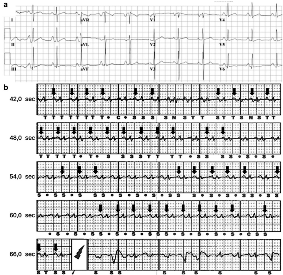
Fig. 1a,b a shows electrocardiogram with atrial enlargement, b arrows indicate all p -waves classified as S or T. S sensing of an event not classified as tachycardia, T sensing of an event classified as tachycardia. dot indicates sensing of an unclassifiable event that is discarded, C indicated capacitor charging and the lightning symbol indicates a shock delivered
