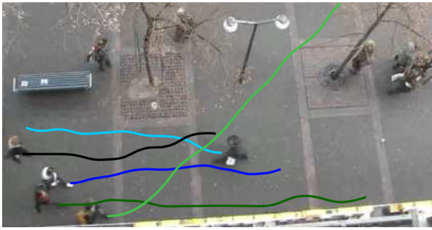
Fig. 6 Environment of the BIWI Walking Pedestrians dataset [62] that served as the basis for the example shown in Fig. 5. Final trajectories of the motion planning in Fig. 5 at t = 11 s are drawn in the scene
