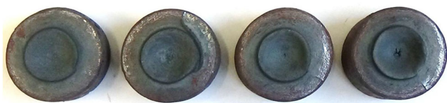
Fig. 5 Deformed specimens obtained from billets (preheated to 1200 °C) at forming lengths ( s ) of (from left to right) 375 mm, 400 mm, 455 mm, and 500 mm
