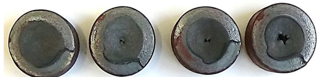
Fig. 4 Deformed specimens obtained from billets (preheated to 950 °C) at forming lengths ( s ) of (from left to right) 150 mm, 175 mm, 200 mm, and 250 mm
