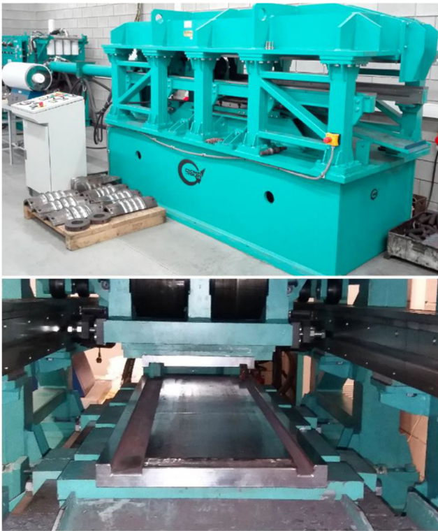
Fig. 2 Laboratory rolling mill used in the tests (top) and a view of workspace adapted for use in the test of rotational compression between channel-dies (bottom)
