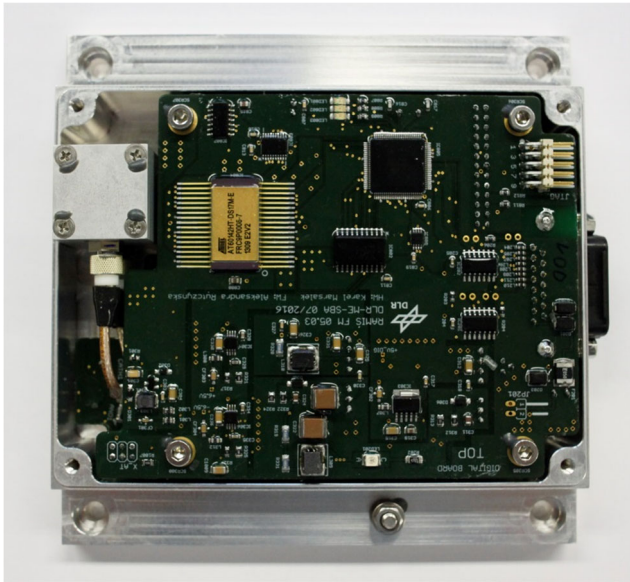
Fig. 3 The Radiation Measurements In Space (RAMIS) Flight Model (FM) detector with open lid showing in the top left part the silicon detector telescope as well as the digital PCB board with the relevant digital electronics. The analogue board with relevant preamplifiers and analogue electronics is below the digital board. In addition one can see on the right part of the outer surface the power and data connector for connection to the Eu:Cropis satellite. Size approx. width 14 cm x height 14 cm x height 4 cm
