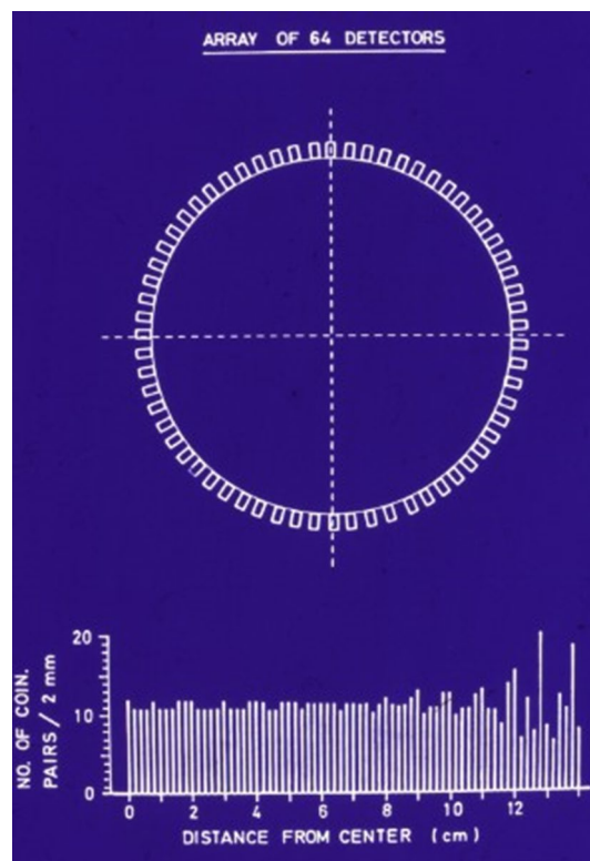
Fig. 8 An array of unequally spaced detectors and the linear sampling density distribution of the array when implemented in the Positologica-I. The figure is courtesy of Dr. Norimasa Nohara
