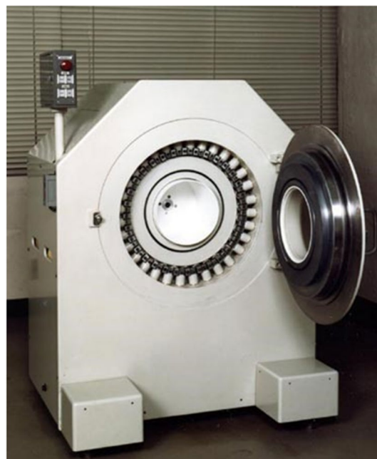
Fig. 7 Positologica-I for human brain studies (© 1979 QST), courtesy of the National Institutes for Quantum Science and Technology
