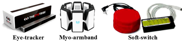
Fig. 6 Commercially available input devices. These devices are used for searching and selection of the items on virtual keyboard application. These devices can be utilized separately and/or in combination with each other to meet the particular needs of the user
