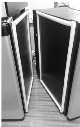
Fig. 10 Sidewalls of the refrigerators equipped with rubber seals
