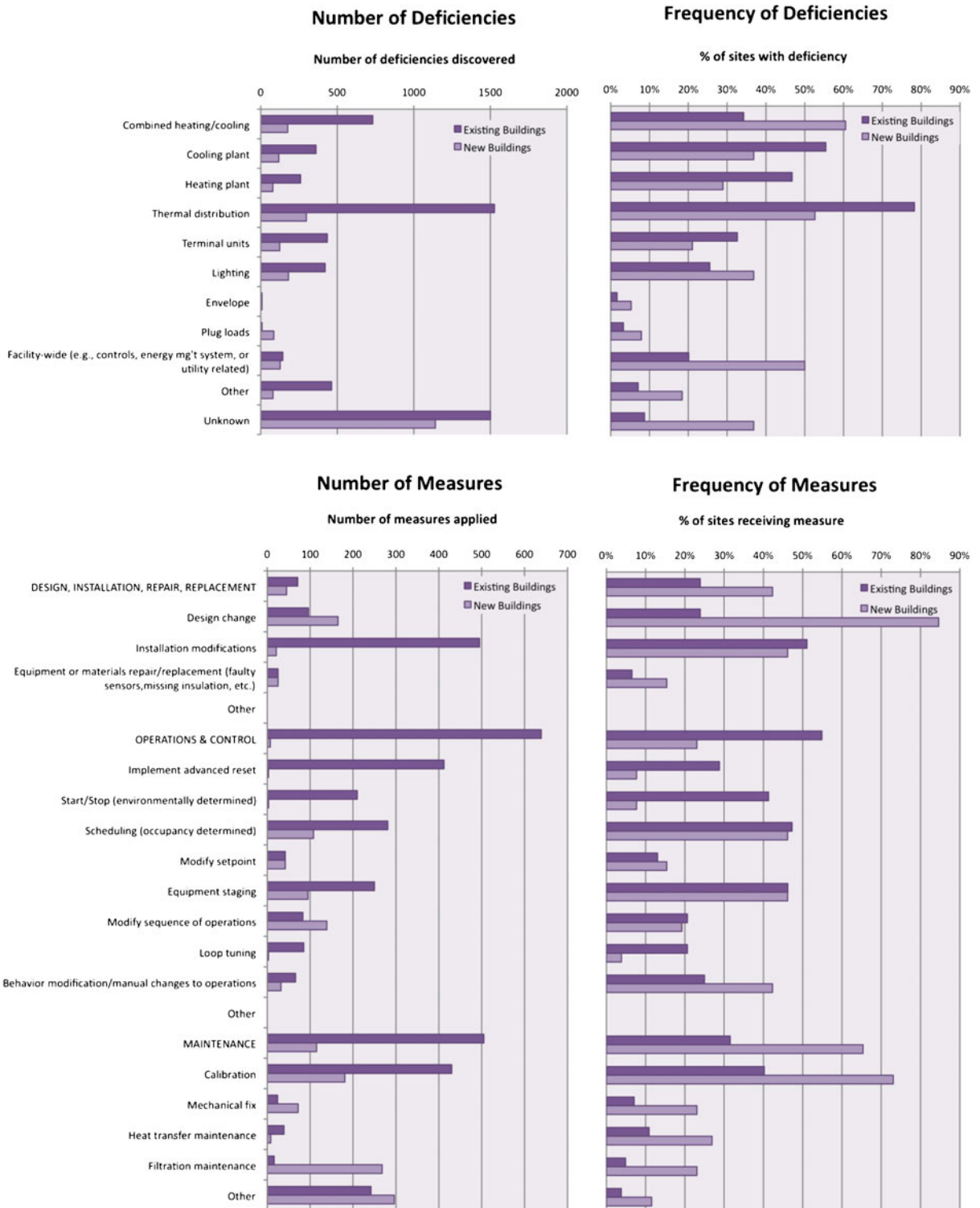
Fig. 4 Types of problems ( Deficiencies ) and their solutions ( Measures )
