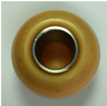
Fig. 1 Photograph of a 32-mm ceramic head (BIOLOX ® forte; CeramTec AG, Plochingen, Germany) with a titanium-alloy sleeve designed to fit the Morse taper of an S-ROM stem (DePuy/J&J, Warsaw, IN, USA).
