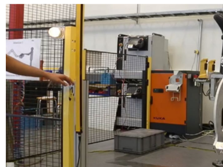
Fig. 5 Engaging the mode-change button after exiting the fenced area
