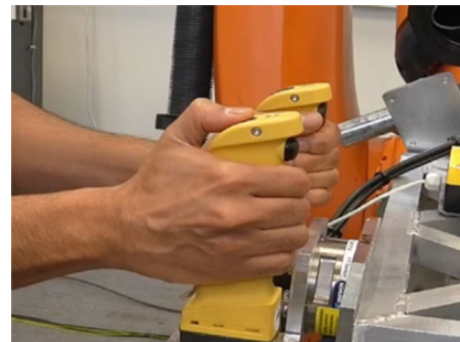
Fig. 4 Initiating the three button switch integrated with the hand-guiding tool
