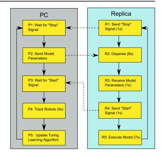
constant duration. The PC also executes a fixed behavioral loop, but the timing is determined by the signals received from the replicas. Therefore, the PC is synchronized with the swarm. The PC communicates with the replicas via Bluetooth. At the start of a run, or after a human intervention (see Sect. 5.3), robots are initially synchronized using an infrared signal from a remote control.
