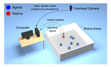
**Fig. 15** Illustration of the general setup for inferring the behavior of physical agents—e-puck robots (not to scale). The computer runs the *Turing Learning* algorithm, which produces models and classifiers. The models are uploaded and executed on the replica. The classifiers run on the computer. They are provided with the agents' and replica's motion data, extracted from the video stream of the overhead camera
