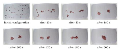
**Fig. 22** Example of collective behavior produced by a model that was inferred by *Turing Learning* through the observation of swarms of physical e-puck robots. A swarm of 40 physical e-puck robots, each executing the inferred model, aggregates in a single spot
