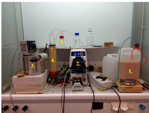
Fig. 3 The experimental apparatus with gas-permeable hydrophobic membrane
