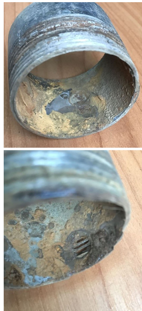
Fig. 1 Macroscopic view of samples of the 60.3-mm pipe
