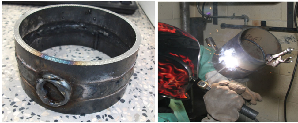
Fig. 12 The author using the SMAW process to generate a multipass weld on a section of pipe in the angular position
