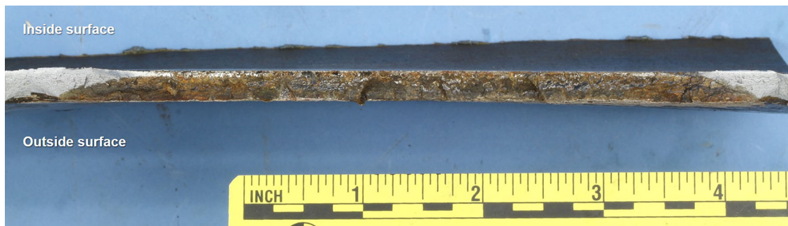
Fig. 4 View of one of the faces of the main crack after laboratory fracture and crack opening
