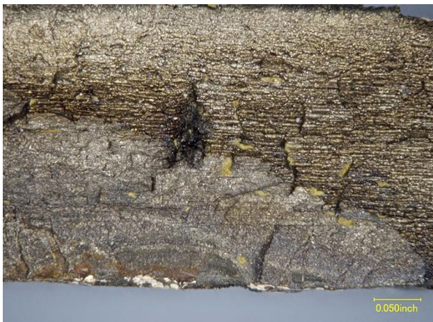
Fig. 5 View of the right edge of the through-wall crack from Fig. 4, showing crack arrest and ratchet marks, consistent with progressive cracking
