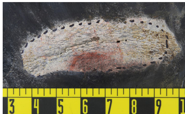
Fig. 3 View of the outside surface of the cracked pipe segment, after sectioning, showing the parallel crack colony about the through-wall crack in the white region
