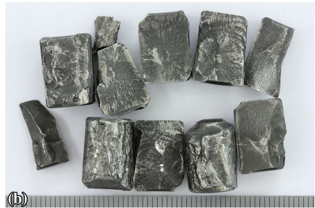
Fig. 8 Overview of rolling elements either intact or catastrophically failed
