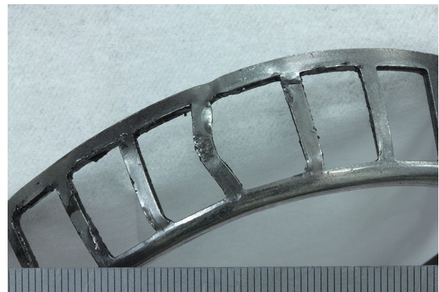
Fig. 7 Fractured cage arm, possibly due to roller seizure
