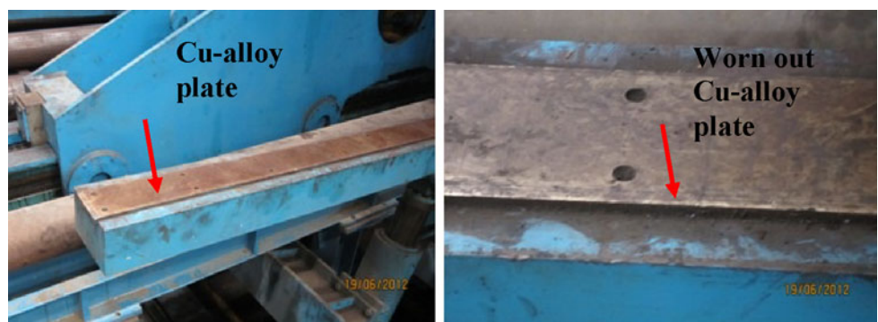
Fig. 10 Cu-alloy plates in wear condition at JCO mill
