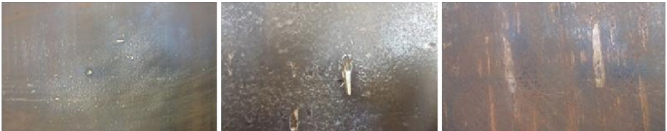
Fig. 9 Golden-yellow color copper-alloy streaks on pipe OD surface
