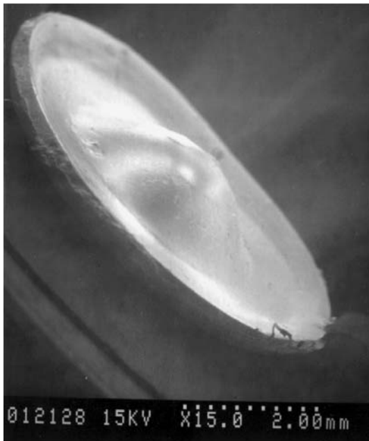
Fig. 16 Pressure relief disk from testing. The taper on the nozzle allowed disk deformation as pressure increased. Note the rolled-up edges. This disk does not rupture at normal operating pressures but distorts to allow air to escape around the nozzle threads
