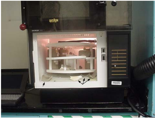
Fig. 1 Interior of microwave after vessel rupture. Parts of the failed vessel remained in the microwave after rupture (shown by arrows) and the vessel carousel was also damaged
