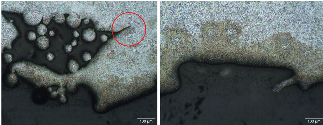
Fig. 12 Optical micrographs of polished and etched cross sections of EBM Ti-6Al-4V with as-built surface (left) and after CAVF (right). The surfaces shown correspond to unsupported horizontal surfaces facing downward in the vertical direction with respect to the EBM growth direction. The circled feature in the left-hand image is inferred to be typical of high stress concentration where fatigue cracks initiate, and is not present after CAVF treatment
