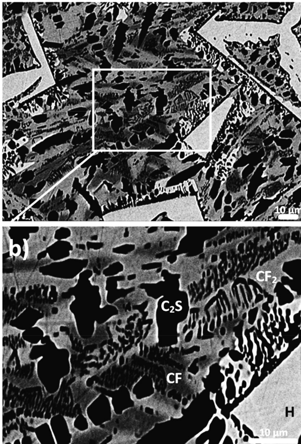
Fig. 4—Example of the complex microstructure formed on cooling from 1623 K to 1073 K (1350 °C to 800 °C), at 2 K/s in air (72.74 wt pct Fe 2 O 3 , 6.11 wt pct SiO 2 and 21.14 wt pct CaO). (H hematite, C 2 S 2CaO·SiO 2 , CF 2 CaO·2Fe 2 O 3 , CF CaO·Fe 2 O 3 ). (b) Detail of (a) (Backscattered electron (BSE) micrographs).
