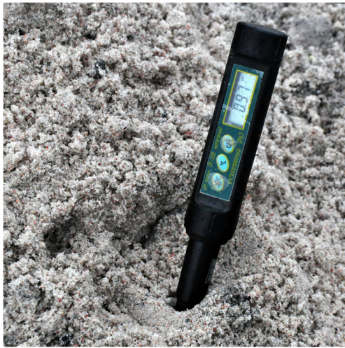
Fig. 5 Extreme soil pH measured within the former “Polchem” area
