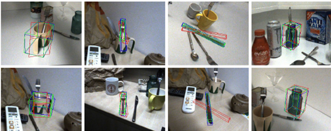
Fig. 11 S^2P^3 qualitative results before and after self-supervision (zoomed-in from Fig. 10). The projected bounding boxes in blue, red and green represent the ground-truth 6D object poses, the results before and after applying self-supervision, respectively
