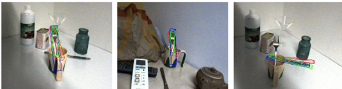
Fig. 13 S^2P^3 qualitative results before and after self-supervision with occlusions (zoomed-in from Fig. 12). The projected bounding boxes in blue, red and green represent the ground-truth 6D object poses, the results before and after applying self-supervision, respectively
