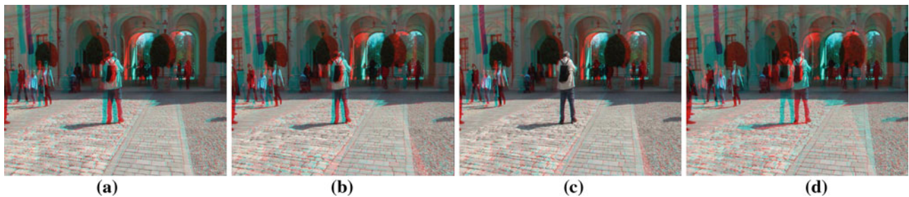
Fig. 6 Changing the target depth range by changing the negative and positive disparity limits: (a) an original stereoscopic frame; (b) target depth range set using \eta_1 = -2^\circ and \eta_2 = 2^\circ ; (c) target depth range set
