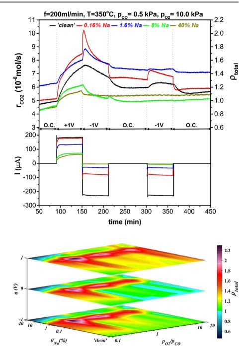
**Fig. 8** Contour map of the overall effect of combined sodium chemical promotion and oxygen ion electrochemical promotion on the catalytic rate of CO oxidation on Pt. The values on the colormap correspond to the total enhancement of the catalytic rate upon polarisation and sodium modification compared to the open-circuit rate for a 'clean' catalyst
