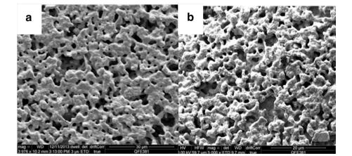
Fig. 2 SEM image of the used Na-modified Pt surface with magnification of  $\times 10,000$  (a) and the corresponding X-ray mapping of Pt (b), O (c) and Na (d)
