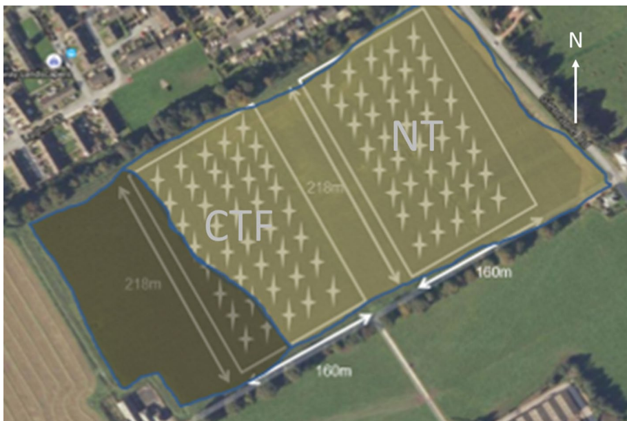
Fig. 3 Sampling points across the NT and CTF plots. The area coloured (light green) is a brown forest soil of the Hollywood association and is imperfectly drained and the area coloured (dark green) is a brown forest soil of the Hollywood association and freely draining (Color figure online)
