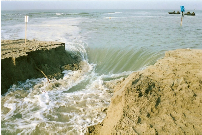
Fig. 1 Photo taken of the breach widening process during the breach experiment in The Zwin, the Netherlands (Visser 1998)
