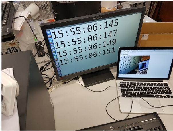
Fig. 5 Picture measuring the capture-render delay
