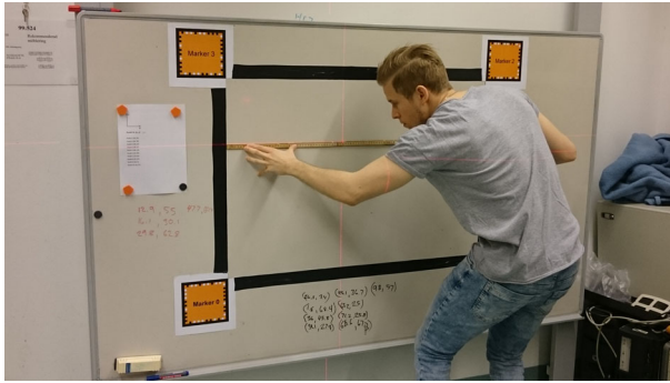
Fig. 7 An experimenter is retrieving the coordinate of a point on the workarea using a ruler and a cross laser pointer
