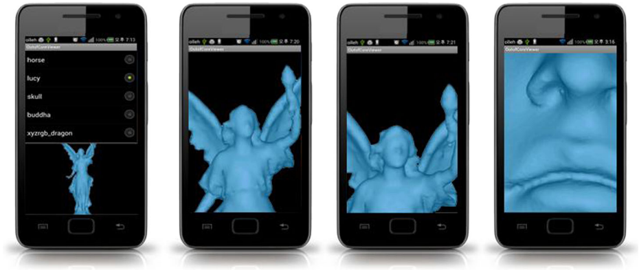
Fig. 18 An example of a hierarchical browsing with a mesh Lucy in our mobile 3D viewer
