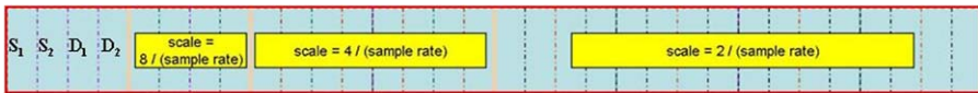
Fig. 1 The structure of the wavelet coefficient vector in Mallat’s algorithm. The second half of the vector contains wavelet coefficients for the scale that is twice the sample spacing. The second quarter of the vector contains those on the scale that is four times larger than the sample spacing. The scale increases in the second eighth to twice that, and so on. The first two components S_1, S_2 contain the so-called “mother function coefficients” (see Press et al. 1992) and the third and fourth ( D_1, D_2 ) are the wavelet coefficients at the coarsest scale (half the length covered by the sample). Higher scales are represented with fewer components
