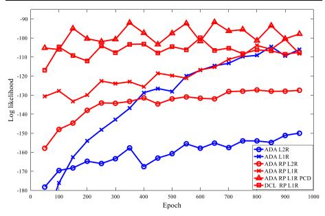
**Fig. 7** Log-likelihood on test set of binarized MNIST for iRBMs with different training strategies. Where "L1R" and "L2R stand for "L1 regularization" and "L2 regularization" respectively, "ADA" stands for "ADA-GRAD", "DCL" stands for "decaying learning rate"
