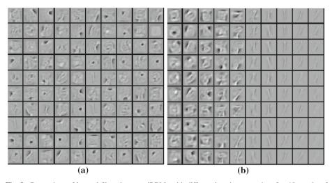
**Fig. 8** Comparison of learned filters between iRBMs with different learning strategies after 10 epochs of training, **a** with RP; **b** without RP. The left-most100 filters are shown starting from the top-left corner and incrementing across rows first
