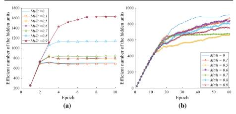
Fig. 4 Growing of iRBMs when using different regrouping rates  $M_t$ , a binarized MNIST; b CalTech101 Silhouettes
