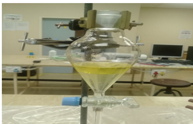
Fig. 1 Experimental setup for the separation of aqueous phase and organic phase
