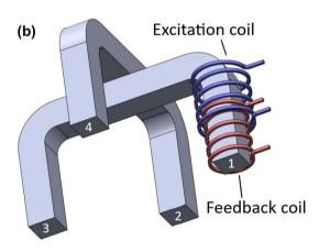
**Fig. 4** Tetrapole probe with **a** four cylindrical poles and **b** orthogonal U-cores with magnetization and feedback coils. Schematic images based on [8]
