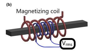
**Fig. 1** Magnetization unit with **a** copper coil wrapped around both legs, schematic image based on [15] and **b** wrapped around the sample, schematic image based on [17]
