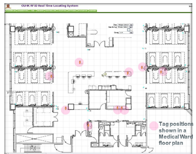
Fig. 1 The RFID-based real-time locating system developed for tracking patient activities
