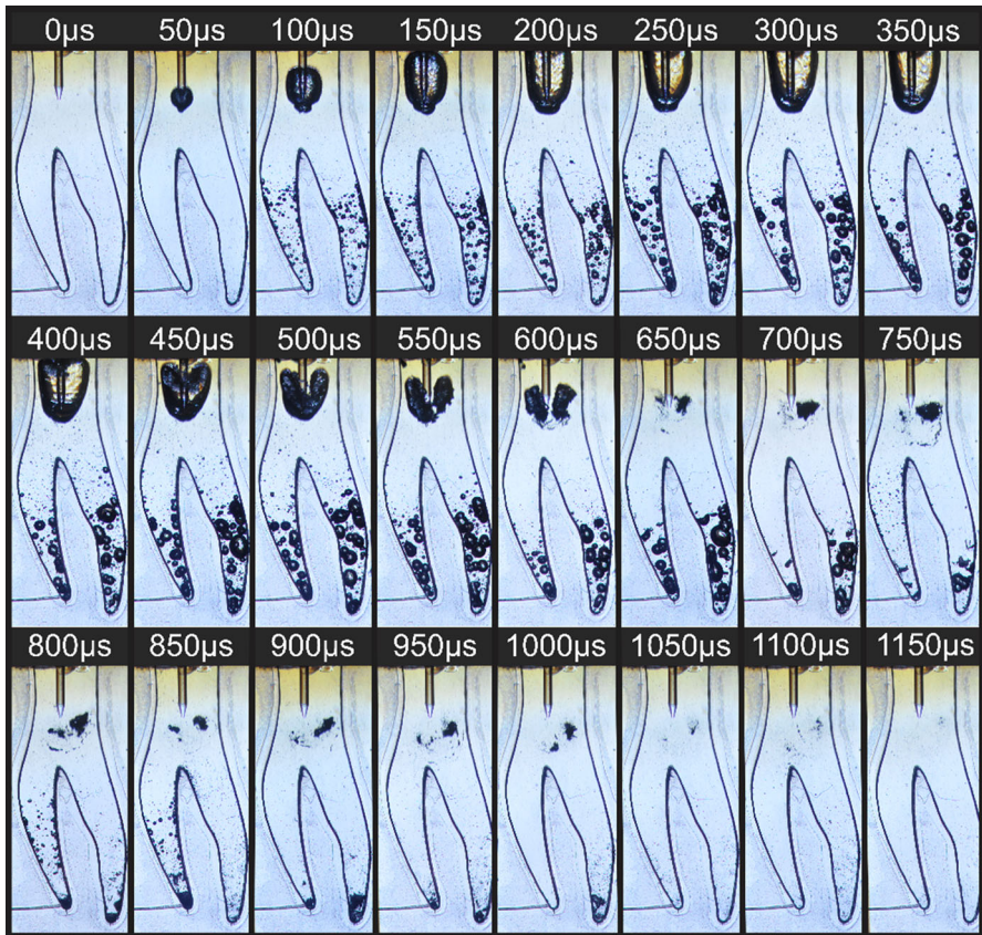
Fig. 2 The series of images shows the life cycle of a laser-induced vapor bubble. Because light of wavelength 2.94\ \mu\text{m} is strongly absorbed in water, a very thin layer of water next to the FT is heated up in a very short amount of time beyond its boiling point. This leads to explosive boiling and a rapid expansion of the cavitation bubble ( 0\ \mu\text{s} to 300\ \mu\text{s} ). This process continues until the pressure inside the bubble is equal to the outside pressure, at which point the bubble starts collapsing ( 350\ \mu\text{s} ). After the initial collapse of the bubble ( 700\ \mu\text{s} ), additional oscillations can occur
