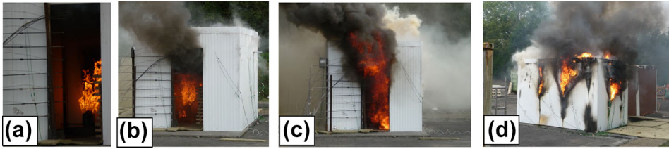
Figure 13. PIR panel enclosure: (a) at ignition; (b) after 8 min; (c) after 22 min; (d) after 24 min.
