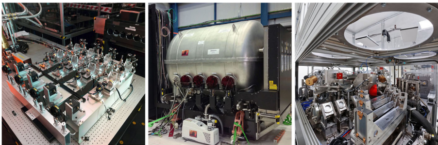
Fig. 2 From 2019 the VLTI interferometric instruments will cover the full atmospheric windows H-band to N-band (1.6–13 \mu\text{m} ): left: PIONIER (H-band; in regular operation), center: GRAVITY (K-band; 2016 in commissioning at the VLTI), right: MATISSE (L, M, N-band; photo taken in the lab; VLTI commissioning will commence in early 2018). Image Credits: ESO, B. Lazareff, MPE/GRAVITY team, MATISSE project, Y. Bresson
