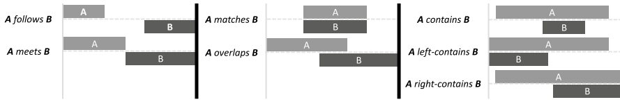
Fig. 1 Seven temporal relation types two event intervals can have, as defined in Allen’s temporal logic (Allen 1983)
