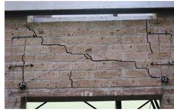
(a) Damage pattern for the masonry wall (from (Augenti et al. 2010) with permission from ASCE); (b) Crack development in the masonry wall (From (Augenti et al. 2010))
